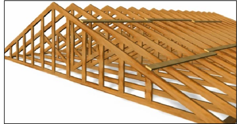
Series of braced trusses
