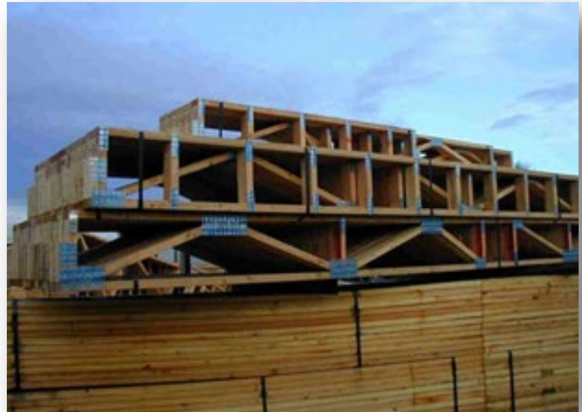
Image of pre-manufactured, parallel chord trusses waiting to be shipped to a jobsite
