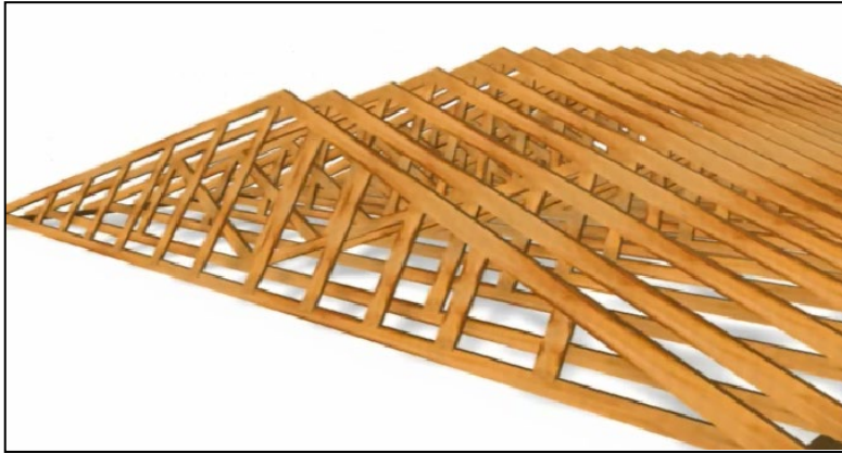
Series of unbraced trusses
